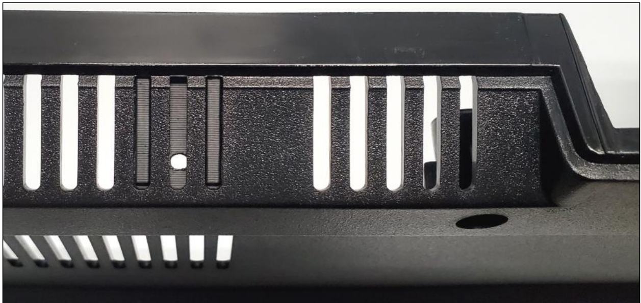
Figure 11b: Single LED mounting bracket placement in lower case housing
