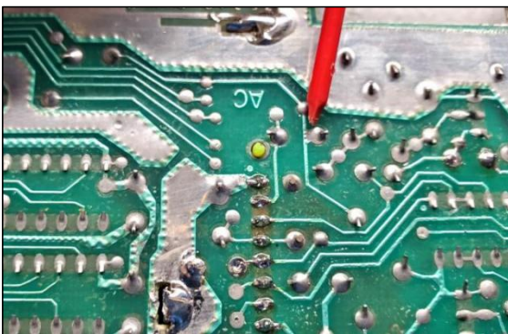
Figure 2a: Audio line to cut
