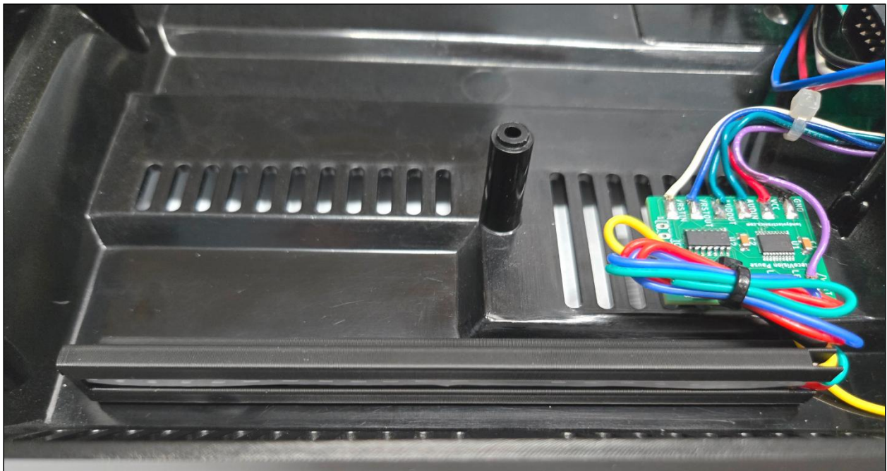
Figure 11d: Dual LED light bar assembly placement in lower case housing
