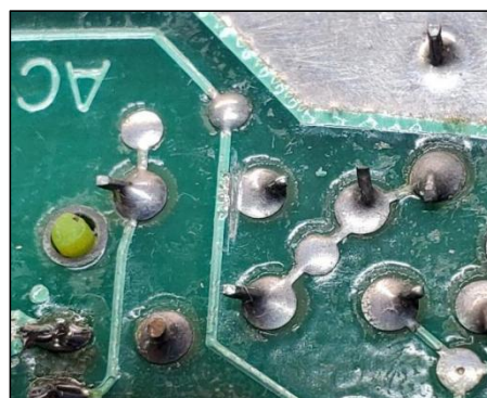
Figure 2b: Audio line cut
