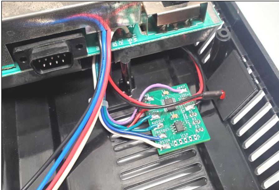
Figure 13: Placement of Pause Mod PCB with single LED assembly
