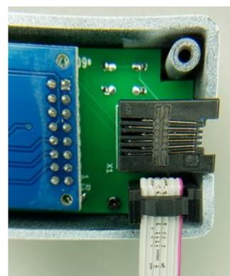
Figure 3: 6-pin Ribbon Cable Attachment
