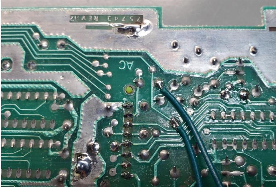
**Figure 3:** Solder two Green wires to audio connections
