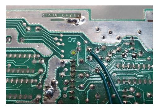
**Figure 3:** Solder two Green wires to audio connections
