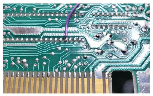
**Figure 6:** Solder Violet wire to Z80 /WAIT connection
