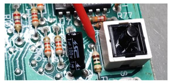
Figure 1: Reset line cut
