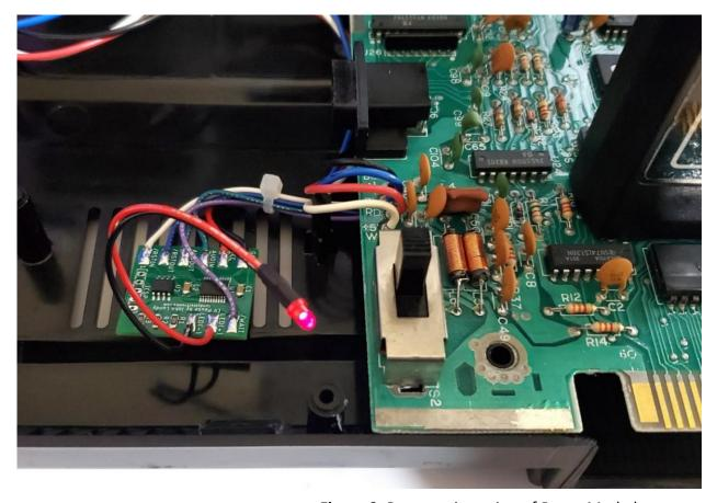
Figure 9: Proper orientation of Pause Mod placement
