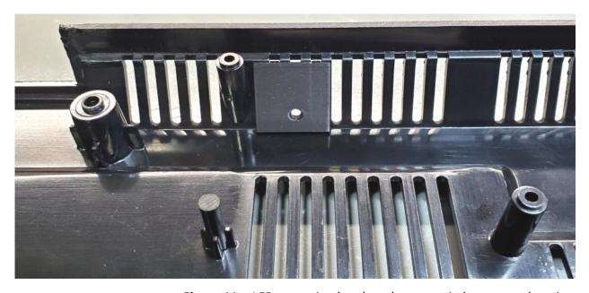
Figure 11a: LED mounting bracket placement in lower case housing
