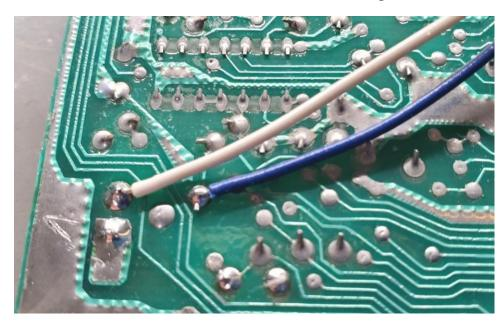
**Figure 4:** Solder White and Blue wires to reset connections
