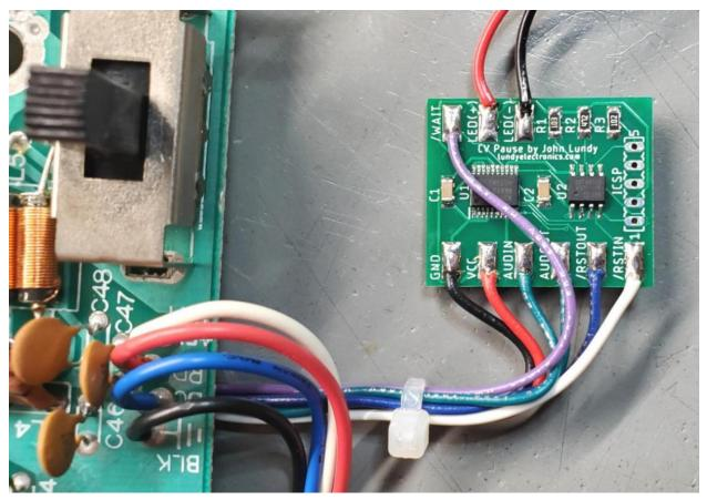
Figure 8: Cleanly trip, strip, and solder wires to the Pause Mod PCB
