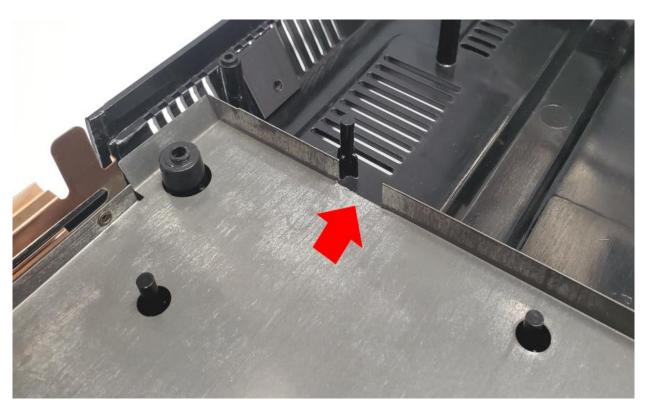
Figure 12: Add notch to lower shield
