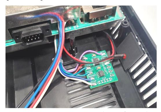
Figure 13: Placement of Pause Mod PCB
