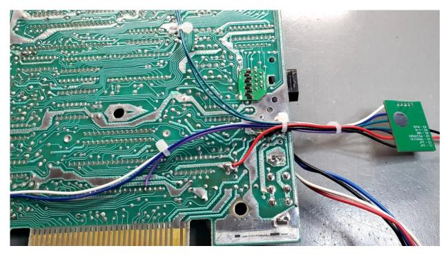
Figure 10: Install wire tie wraps
