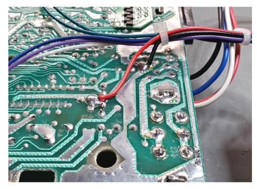
Figure 5: Solder Red and Black to power connections
